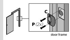
**B** Are the latch holes centered in the door hole?
