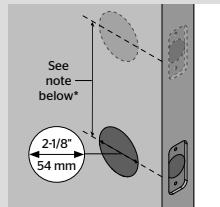
**B** Measure to confirm that the backset is either 2-3/8" or 2-3/4" (60 or 70 mm).
