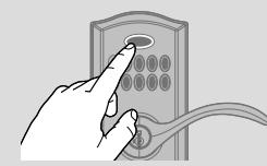
**E** Enter a Programming Code. It must be between 4 and 8 digits. The Programming Code cannot be the same as any user code.
