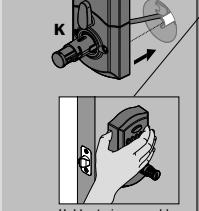
Ensure both interior and exterior assemblies are parallel to edge of door before securing.
