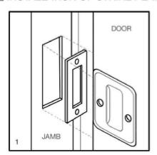
Mark and mortise strike on jamb to correspond to lock position on door 1 1/16" x 2 1/2" x 1/16" deep.
